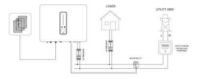
Figure 5-2 Electrical wiring diagram of export limit
