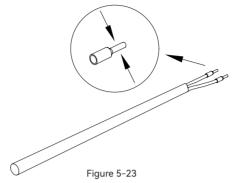
④ Insert the stripped end of the three wires into the appropriate hole of the terminal head. Please try to pull out the cable to make sure it is well connected.
