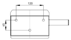
Figure 4-4 Dimensions of wall bracket
