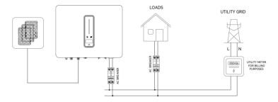
Figure 5-1 Electrical wiring diagram
