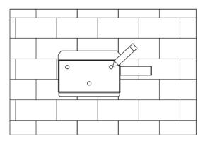
Figure 4-5 Marking hole position using installation bracket
