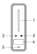
Figure 3-4 Inverter display interface
