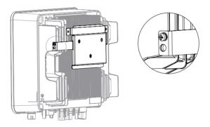
Figure 4-7 Mounting the inverter
