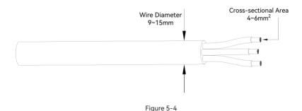
AC output side uses a three-core cable (L, N, and PE).
