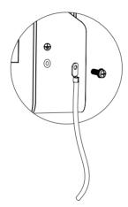
Figure 4-8 Grounding terminal connection
