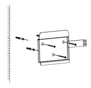
Figure 4-6 Fixing the wall bracket
