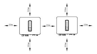
Figure 4-2 Recommended installation spacing
