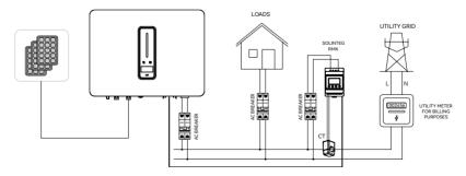
Figure 5-3 Electrical wiring diagram of export limit & 24 hours load consumption
