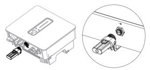
Figure 5-18 Monitoring device installation
